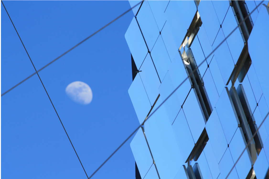
Figure 2.7: Close-up of some MAGIC-I mirrors at the edge of the reflector. Most of them are of an older kind, and consist of four 0.25\text{ m}^2 sub-units. Two new generation mirrors are visible at the bottom and at the top right corner. They have no subunits. (G. Ceribella / MPI)
