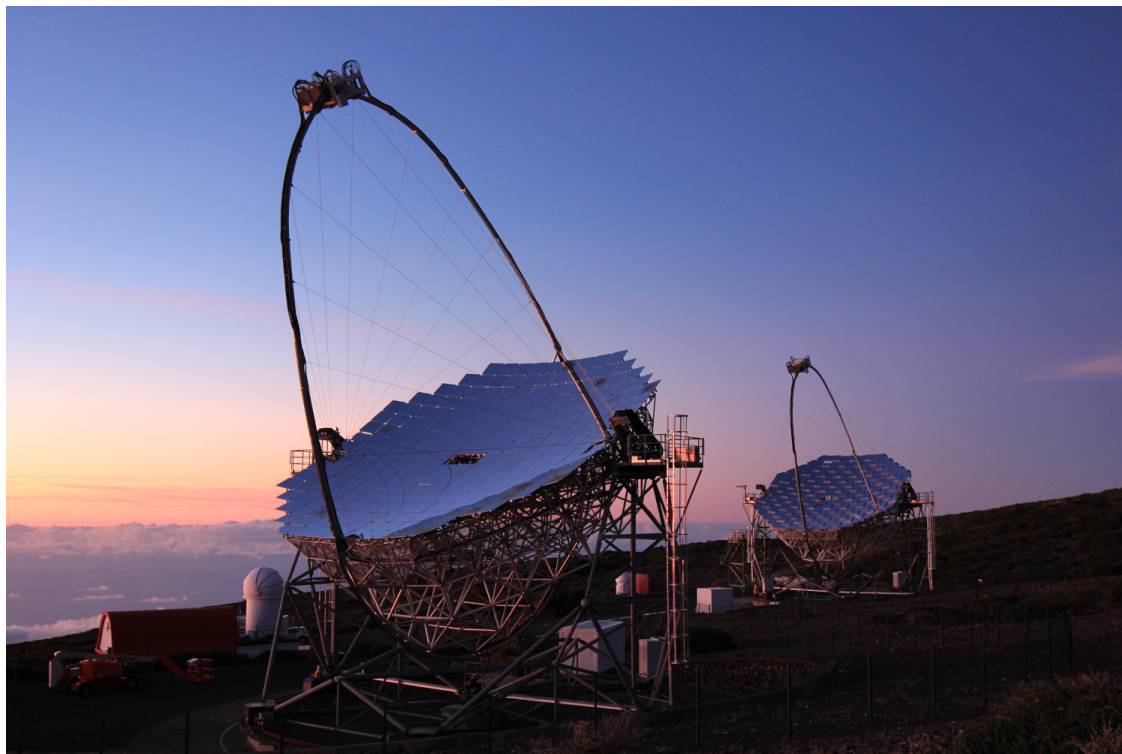
Figure 2.6: Picture of the MAGIC Telescopes at the beginning of the evening operations. MAGIC-II is in the foreground and MAGIC-I is in the background. The roof of the counting house and the small dome of the MAGIC LIDAR are visible in the lower left corner. (G. Ceribella / MPI)
