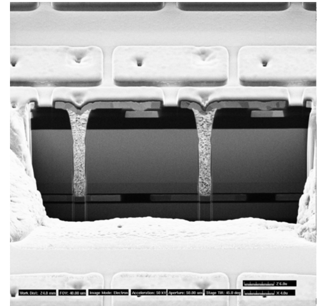
Fig.: Cross section of a vertically integrated test chip structure, showing 2.5 x 2.5 μm 2 interchip vias (FIB)
