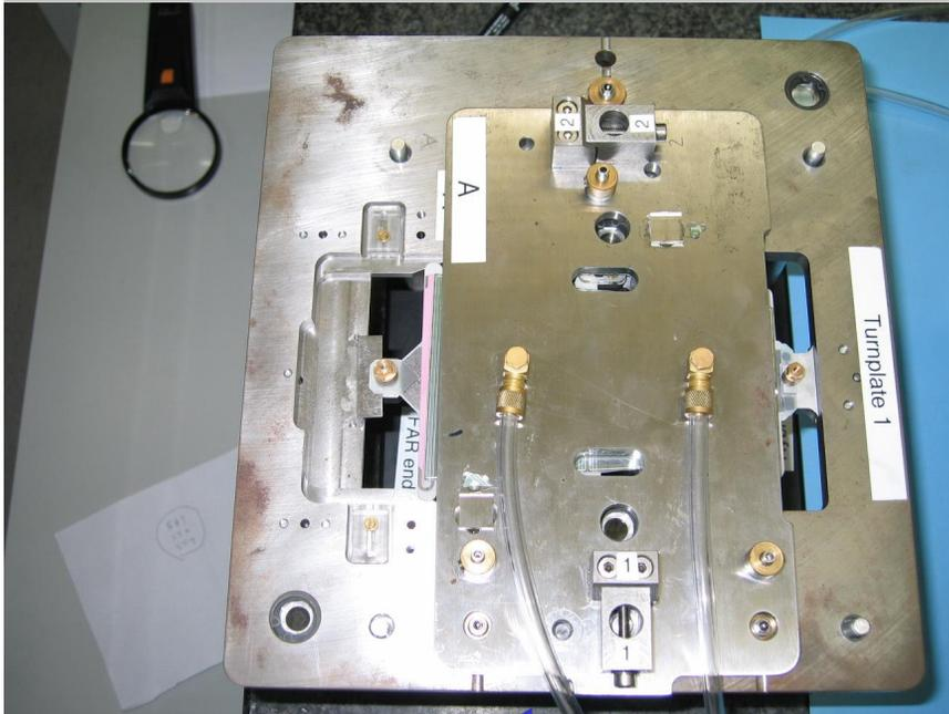
assembled sandwich of spine and sensors
