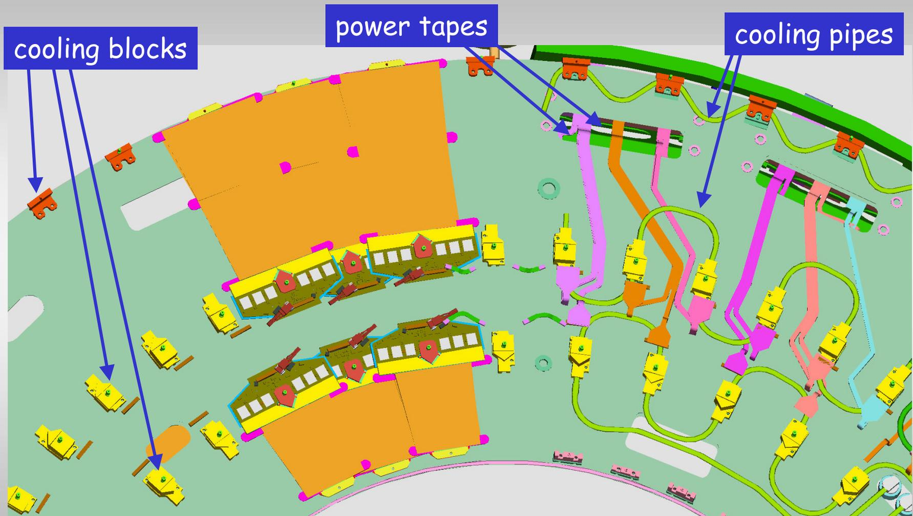
middle modules are mounted on the backside of the disc
