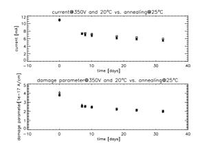
Fig. 3. Annealing of the current and the damage parameter  $\alpha$  for 24 GeV/c protons.
