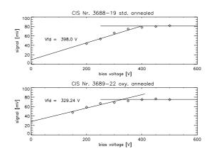
Fig. 6. Signal versus bias voltage for the detectors on standard and oxygenated material after 32 days annealing at  $25^{\circ}$  C.
