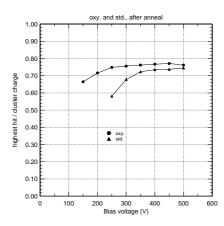
Fig. 7. Fraction of the charge in the highest hit versus the bias voltage after long term annealing
