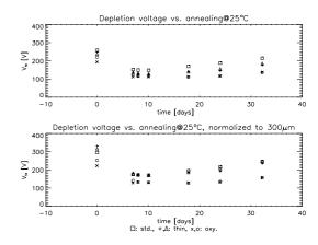
Fig. 4. Development of the full depletion voltage with annealing time.
