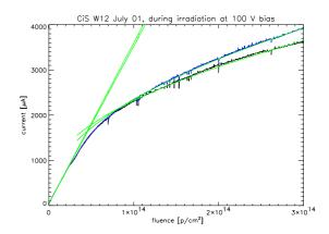
Fig. 1. Currents of two detectors during irradiation normalized to  $20^{\circ}C$  together with the fit results. The lower curve is the standard detector, the upper curve the oxygen enriched one (see text).
