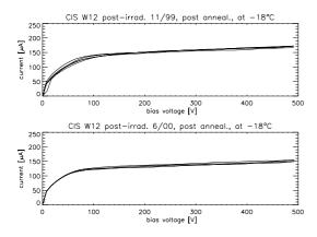
Fig. 2. IV curves one detector on standard, two on standard thin and two on oxygen enriched material (upper plot), and of four detectors, all on oxygen enriched material (lower plot), after two different irradiations to the same nominal fluence and 7 days annealing at  $25^{\circ}C$ .
