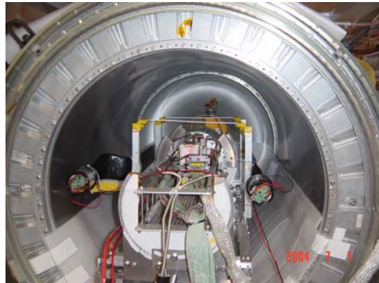
Fig. 2. The chamber inside the 1 T PCMag at KEK.
